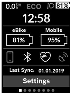
As well as the status bar, the status page also shows you the current time and the state of charge of all your eBike's batteries, as well as the state of charge of your smartphone battery if the smartphone is connected via *Bluetooth*<sup>®</sup>.
