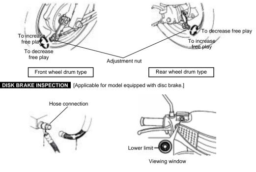
Visual Inspection for leakage or damage. If there is any, take your scooter to SYM Authorized Dealer or Franchised Dealer for a check or repair.
