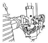
4. Pull the choke lever up (choke valve closed position)
