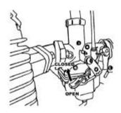
4. Pull the choke lever up (choke valve closed position) The choke lever is below the carburetor left side.
