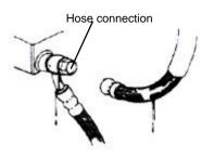
( leak, damaged, looseness of brake line )
