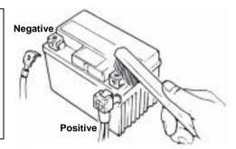
This scooter is equipped with a maintenance-free type battery, so it is unnecessary to check and add electrolyte. Have your scooter checked by SYM Authorized Dealer or Franchised Dealer should any abnormality is found.
