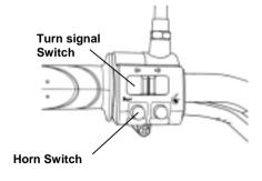
Turn the ignition switch key "\tilde{\cappa}", and press horn button down, if the horn does not sound, the fuse may have been blown.
